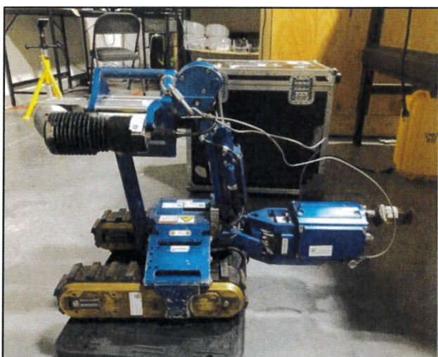
Figure 11. The Versatrax 150 CCTV crawler with the Spectrum 90 Camera prior to the start of inspections.
