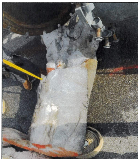
Figure 7. After being removed from the transmission main, the first pig showed significant damage, with large chunks of foam missing from the front/leading end. The foam was removed by hand out of the strainer by CP Construction personnel.
